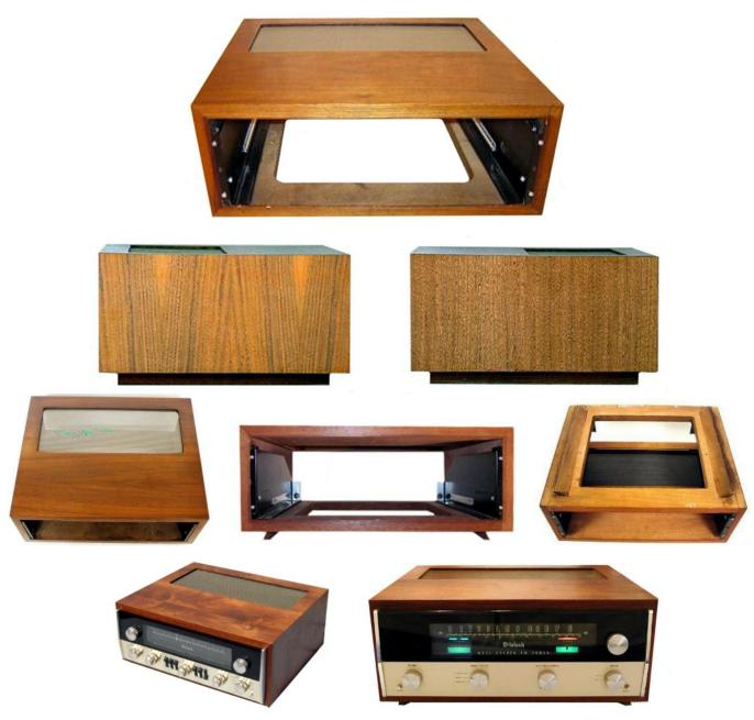
Oiled or urethane walnut veneer on plywood. For 5-7/16" high front panel. Recessed metal vent grille. ¾" Wood wedge rails. Used originally with C 28, C 27, C 26, C 32, MR 73, MR 77, MX 112, MX 113, MX 114, MX 115, MI 3, MC 2505 and MC 2125. Also fits MA 5100. Can be used with same models as the earlier L 11 and later L 52 and L 62 cabinet.
