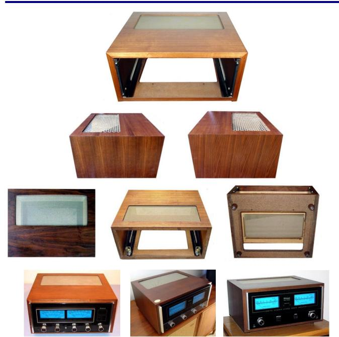
Lacquered walnut on particle board. For 7-1/8" high front panel – earlier, narrow models. Recessed metal vent grille. Plastic feet. For MC 2255, MC 2002, MC 7200(N), MC 7270, and MC 7300(N). Also fits non-Panloc MC 2200 and MC 2250. Can be used with same models as the earlier L 14 cabinet and later L 62 cabinet. Model L 54A was identical but has a flush metal grille.
