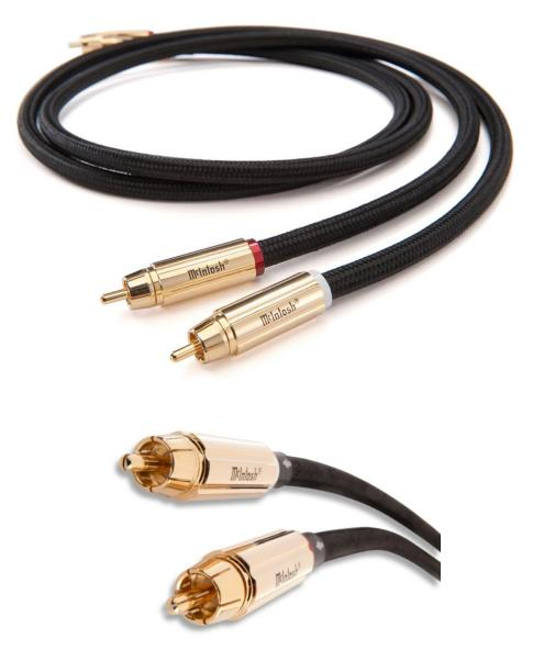
SPECIFICATIONS: Conductor Configuration: Twisted pair. Conductor Gauge and Material: 22 AWG PCOCC. Insulation: Low density polyethylene. Shielding: Copper foil + 95% coverage copper braid. Outer Jacket: PVC Jacket with black nylon webbing. Termination Connector: Gold plated brass RCA male. Outside Cable Dimension: 8.5mm. Unique Features: Directional arrows to sync device, shields grounded at source ends only.
