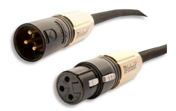
SPECIFICATIONS: Conductor Configuration: Twisted pair and ground. Conductor Gauge and Material: 22 AWG PCOCC. Insulation: Low density polyethylene. Shielding: Copper foil + 95% coverage copper braid. Outer Jacket: PVC Jacket with black nylon webbing. Termination Connector: Gold plated brass XLR male. Outside Cable Dimension: 9mm. Unique Features: Separate signal ground from chassis ground.
