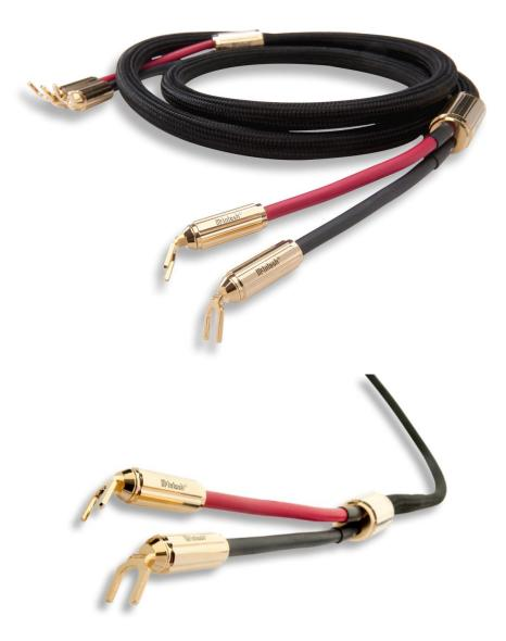
SPECIFICATIONS: Conductor Configuration: Multiple conductors and gauges. Conductor Gauge and Material: 9 AWG PCOCC. Insulation: Polyethylene foamhigh voltage. Shielding: N/A. Outer Jacket: PVC UL CL2 jacket with black nylon webbing. Termination Connector: Gold plated brass spade. Outside Cable Dimension: 15.8mm. Unique Features: Gold plated brass breakout fittings.
