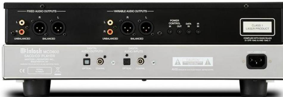
**BACK PANEL:** **FIXED L & R AUDIO OUTPUTS:** UNBALANCED and BALANCED. **VARIABLE L & R AUDIO OUTPUTS:** UNBALANCED and BALANCED. **POWER CONTROL:** IN and OUT. **DATA control IN.** **IR:** sensor input. **DIGITAL AUDIO OUTPUTS:** OPTICAL and COAXIAL. **DIGITAL AUDIO INPUTS:** OPTICAL and COAXIAL. Power cord receptacle.
