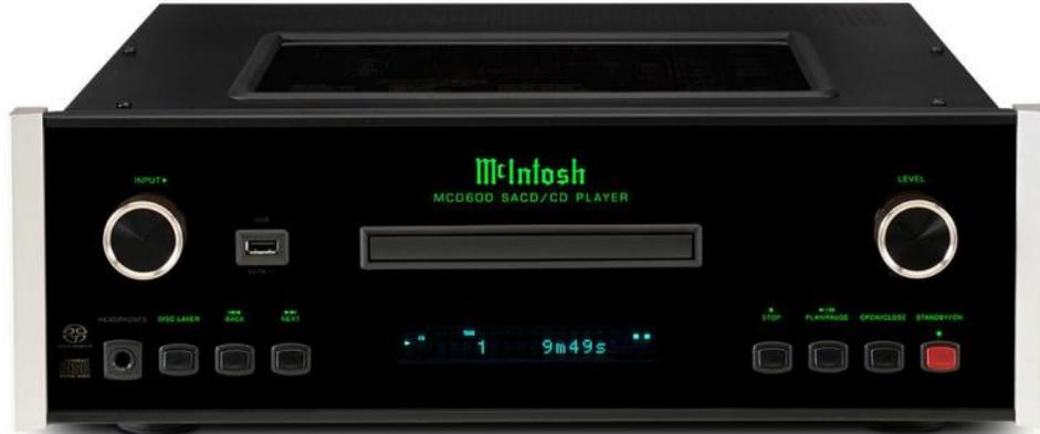
**FRONT PANEL:** Glass with LED/fiber-optic illuminated green nomenclature. **INPUT** control. USB input. Disc tray. IR remote sensor. **LEVEL/MUTE** control (with indicator). 1/4" **HEADPHONES** jack. Touch buttons: **DISC LAYER**, track: **BACK**, **NEXT**. Digital display. Touch buttons: **STOP** (with indicator), **PLAY/II PAUSE**, **OPEN/CLOSE**, **STANDBY/ON** (with indicator).
