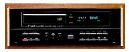
FRONT PANEL: Glass with gold nomenclature and anodized black aluminum panel. Disc drawer. IR REMOTE SENSOR. DAMAGED DISC/MUTE indicator. Digital display.
