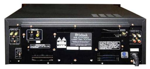
BACK PANEL: Composite VIDEO OUT: 1 and 2. S-VIDEO OUT: 1 and 2. OPTICAL DIGITAL OUT.
