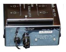
**SIDE PANEL:** LEFT and RIGHT INPUT. LEFT and RIGHT OUTPUT. EQUALIZER MODE switch: IN or OUT. Other side: Power cord. FUSE.
