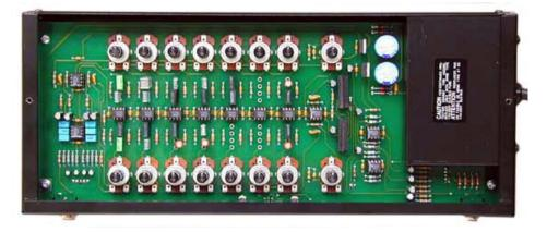
**TOP PANEL:** (under) removable cover: 7 programmable boost or cut filters per channel. Filter frequency and width can be selected with plug-in capacitors. Separate controls for amplitude of each filter. Separate left and right high frequency compensation controls.
