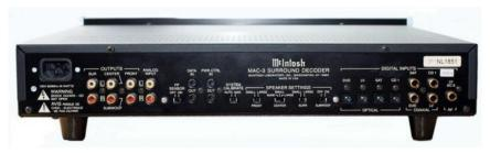
BACK PANEL: Power cord receptacle. OUTPUTS: Left SURROUND, CENTER, Left FRONT, Right SURROUND, SUBWOOFER, Right FRONT. Left & Right Analog Input. FP SENSOR Switch: OFF OR ON. DATA IN and OUT. POWER CONTROL IN and OUT. SYSTEM CALIBRATE Switch: AUTO OR MAN. SPEAKER SETTINGS SWITCHES: FRONT: SMALL OR LARGE, CENTER: NONE, SMALL OR LARGE, SURROUND: SMALL OR LARGE, SUBWOOFER: OFF OR ON. DIGITAL OPTICAL INPUTS: DVD, LV, SAT, CD 1. DIGITAL COAXIAL INPUTS: SAT, CD1, DVD, LV. LV RF AC-3 INPUT.
