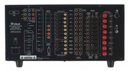
BACK PANEL: FUSE. Power cord receptacle. COMPONENT VIDEO INPUTS 1 and 2: Y, PR and PB. Zone A monitor COMPONENT VIDEO OUTPUTS: Y, PR and PB. KEYPAD connectors: ZONE A and B. IR INPUTS: IR POWER Switch: OFF or ON, inputs for ZONE A and ZONE B. POWER CONTROL out for ZONE A and ZONE B, ACCESSORY, and VIDEO. DATA ports for TUNER, AUX, CD, SAT, TV, DVD, VCR 1, VCR 2, HOME, SUM, SUM A. Optical DIGITAL INPUTS: CD 1, SAT and LV. Coaxial DIGITAL INPUTS: AUX, CD and SAT.
