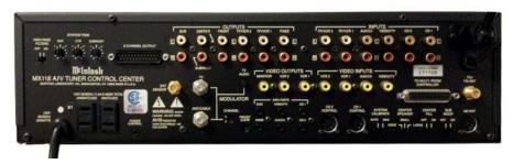
(EARLY) BACK PANEL: SYSTEM TRIM controls: HIGH PASS FILTERS switch: OFF OR ON.
