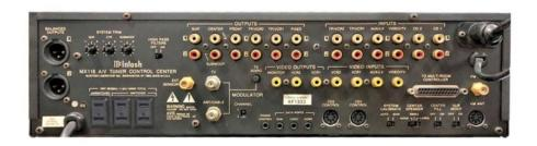
(LATE) BACK PANEL: BALANCED OUTPUT XLR connectors L & R. SYSTEM TRIM controls: SURROUND, CENTER, SUBWOOFER. HIGH PASS FILTERS SWITCH: OFF OR ON. OUTPUTS: L & R SURROUND, CENTER & SUBWOOFER, L & R FRONT, L & R TP/VCR2, L & R TP/VCR1, L & R FIXED. INPUTS: TP/VCR2, TP/VCR1, AUX/LV, VIDEO/TV, CD 2, CD 1. Built in AM loopstick antenna.
