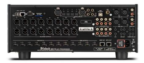
BACK PANEL: USB 1 and 2 connector. NET 1 LAN connector. RS232 control connector. PROCESSOR SD CARD Slot. MICrophone input. DIGITAL INPUTS: 1 through 4 (optical), 5 (balanced), 6 through 8 (coaxial). ZONE OUTput. USB 3 PC AUDIO INPUT. Ground connector. BALanced audio INput: Left & Right 1. Left & Right PHONO inputs.
