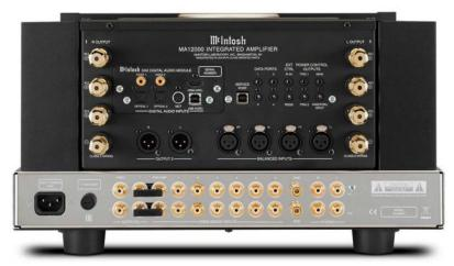
BACK PANEL: Right speaker OUTPUT connectors for 8, 4 and 2 OHMS. DA 2 DIGITAL AUDIO MODULE: DIGITAL AUDIO INPUTS: OPTICAL 1, OPTICAL 2, MCT, HDMI, USB AUDIO. SERVICE PORT. DATA PORTS: 1, 2, 3, 4. EXTERNAL CONTROL: IR IN / RS232. POWER CONTROL OUTPUTS: TRIG 1 / TRIG 2, MAIN / PASSTHRU INPUT. Left speaker OUTPUT connectors for 8, 4 and 2 OHMS.
