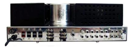
**BACK PANEL:** FUSE. Power cord. AC OUTLETS: 1 unswitched, 3 switched. LEFT & RIGHT SPEAKER output barrier strips (early units had two vertical terminal strips – late units had a single horizontal terminal strip). L+R GAIN CONTROL. Ground binding post. L+R output. TAPE OUTPUTS. INPUTS: TAPE MON, AUX, TAPE, TUNER, PH 1, PH 2, TAPE HEAD.
