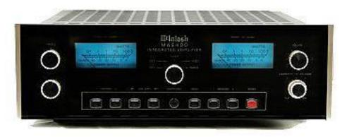
FRONT PANEL: Glass with illuminated teal/gold nomenclature. TREBLE. Left POWER OUTPUT meter (linear WATTS or DECIBELS). POWER GUARD light. INPUT SELECTOR: CD 1, CD 2, TUNER, VIDEO and PH/AUX. Right POWER OUTPUT meter (linear WATTS or DECIBELS). POWER GUARD light. VOLUME. Mute light. With indicator lights: TAPE MON 1, TAPE MON 2, TAPE COPY: 1►2 and 2►1. HEADPHONES jack. Pushbutton switches with indicator lights: MONO, SPEAKERS: 1 and 2, and POWER. Concentric BALANCE: Ltor / LOUDNESS: FLAT to MAX.
