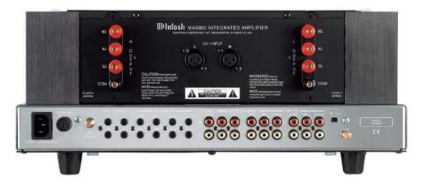
BACK PANEL: Right speaker OUTPUT connectors for 2, 4 and 8 OHMS. Balanced CD 1 INPUTS. Left speaker OUTPUT connectors for 2, 4 and 8 OHMS. Power cord receptacle. FUSE. Coax external Sensor connector. POWER CONTROL connectors: MAIN, ACCESSORY, POWER CONTROL 1 and 2. DATA PORTS: VIDEO, TAPE, TUNER, CD 2, CD 1, AUX, HOME. Jumper: OUTPUTS 1, POWER AMP INPUT. OUTPUTS 2. TAPE OUTPUTS. Inputs: TAPE, VIDEO, TUNER, CD 2, AUX/PH. Selector switch: AUX or PH. Ground binding post.
