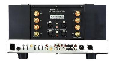
BACK PANEL: Right speaker OUTPUT connectors for 2, 4 and 8 OHMs. Balanced CD 1 and DVD INPUTS. Left speaker OUTPUT connectors for 2, 4 and 8 OHMs. ← Power cord receptacle. FUSE. POWER CONTROL connectors: MAIN, ACCESSORY, POWER CONTROL 1 and 2. Coax External SENSOR connector. DATA PORTS: CD1, SERVER, CD 2, REC, DVD, TUNER. Input: PHONO. Ground binding post. Inputs: CD 2, SERVER, REC, TUNER, Jumper: POWER AMP INputs. OUTPUTS: POWER AMP OUTPUTS 1, REC, balanced OUTPUTS 2.
