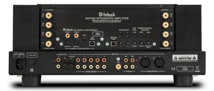
BACK PANEL: Right speaker OUTPUT connectors for 8, 4 and 2 OHMS. DA 1 DIGITAL AUDIO MODULE: DIGITAL AUDIO INPUTS: COAX 1, COAX 2, / OPTICAL 1, OPTICAL 2, MCT digital audio input, USB AUDIO. SERVICE PORT. DATA PORTS: 1, 2, 3, 4. EXTERNAL CONTROL: IR IN / RS232. POWER CONTROL OUTPUTS: TRIG 1 / TRIG 2, MAIN / PASSTHRU INPUT. Left speaker OUTPUT connectors for 8, 4 and 2 OHMS.
