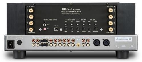
BACK PANEL: Right speaker OUTPUT connectors for 2, 4 and 8 OHMS. DIGITAL AUDIO INPUTS: DIG 2 (coaxial), DIG 2 (optical), USB-D/A. DATA PORTS: DVD / SERVER, CD / CD2, TUNER / AUX. EXTERNAL CONTROL: IR IN / RS232-C. POWER CONTROL: TRIG 1 / TRIG 2, MAIN / PASSTHRU. Left speaker OUTPUT connectors for 2, 4 and 8 OHMS.
