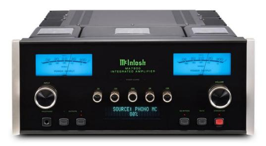
FRONT PANEL: Glass with LED/fiber-optic illuminated green nomenclature. Left POWER OUTPUT meter (LINEAR WATTS OR DECIBELS). Left and right POWER GUARD lights. Right POWER OUTPUT meter (LINEAR WATTS OR DECIBELS).
