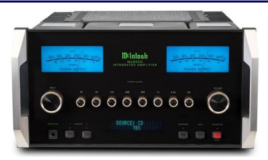
FRONT PANEL: Glass with LED/fiber-optic illuminated green nomenclature. Left POWER OUTPUT meter (LINEAR WATTS Or DECIBELS). Left and right POWER GUARD lights. Right POWER OUTPUT meter (LINEAR WATTS Or DECIBELS).
