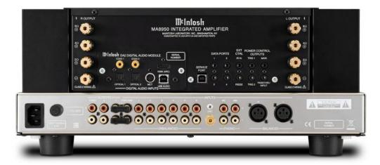
BACK PANEL: Right speaker OUTPUT connectors for 8, 4 and 2 OHMS. DA 2 DIGITAL AUDIO MODULE: DIGITAL AUDIO INPUTS: COAX 1, COAX 2. HDMI (ARC) / OPTICAL 1, OPTICAL 2, MCT digital audio input, USB AUDIO. SERVICE PORT. DATA PORTS: 1, 2, 3, 4. EXTERNAL CONTROL: IR IN / RS232. POWER CONTROL OUTPUTS: TRIG 1 / TRIG 2, MAIN / PASSTHRU INPUT. Left speaker OUTPUT connectors for 8, 4 and 2 OHMS.
