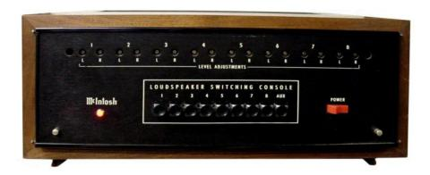
FRONT PANEL: Brushed black anodized aluminum. LEVEL ADJUSTMENTS pots for Left and Right speakers 1 through 8 (behind removable panel).
