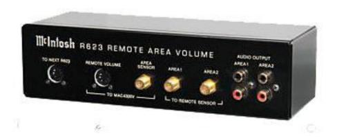
FRONT PANEL: TO NEXT R623 DIN Connector. TO MAC4300V REMOTE VOLUME DIN connector / AREA SENSOR COAX connector. TO REMOTE SENSOR: AREA 1 and 2 COAX connectors. AUDIO OUTPUT: left and right AREA 1 and AREA 2.
