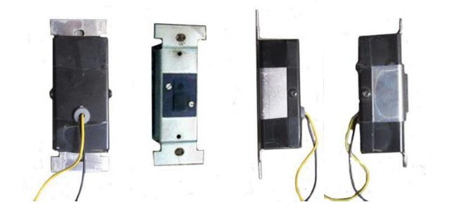
The **R 649** is a wall mounted IR sensor that fits in a single gang wall switch box. It includes a RED LED that indicates when the area is ON, and blinks when the area is muted. It is connected to the master control unit with a single RG6 or RG59U coax cable.
