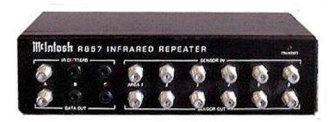
FRONT PANEL: IR EMITTERS coax, data input. / DATA OUT coax, data output. SENSOR INputs: MAIN, 1, 2, 3, 4, 5 / SENSOR OUTputs: MAIN, 1, 2, 3, 4, 5.
