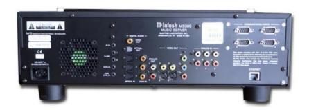
BACK PANEL: Power cord receptacle. Inputs: IR sensor INput, S-LINK, DATA IN, POWER CONTROL IN. ✓ DIGITAL AUDIO: COAX OUT, OPTICAL OUT, OPTICAL IN: 1,2 & 3. COAX IN: 1,2 & 3. ✓ Left and Right AUDIO OUTputs. ✓ VIDEO OUTputs: Composite (2), s-video (2), component video output: Y, CB and CR. ✓ Left and Right AUDIO INputs (3). ✓ RS232 COMMUNICATION PORTS (4). ✓ ETHERNET port.
