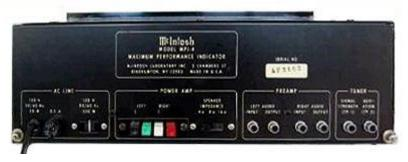
**BACK PANEL:** Power cord. FUSE. Unswitched AC outlet. POWER AMP: Push terminals for: LEFT and RIGHT speaker inputs. SPEAKER IMPEDANCE switch:  $4\,\Omega$ ,  $8\,\Omega$  or  $16\,\Omega$ . PREAMP: LEFT AUDIO INPUT, LEFT AUDIO OUTPUT, RIGHT AUDIO INPUT, RIGHT AUDIO OUTPUT. TUNER: SIGNAL STRENGTH (TP 1), DEVIATION (TP 2). Panloc mounting.
