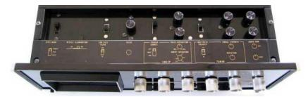
**TOP PANEL:** LEVEL MODE: NORMAL, PEAK, RESET. RETICLE ILLUMINATION: OFF OR ON. LOW PASS FILTER: OUT OR IN. FOCUS. SWEEP: TRIGGER SOURCE: LEFT, RIGHT, LINE, TRACE SEPARATION: MIN to MAX, SWEEP EXPANSION: 0.25 to 5. TUNER: MULTIPATH POLARITY + Or -, SIGNAL STRENGTH, DEVIATION. AUDIO TRIM: LEFT and RIGHT.
