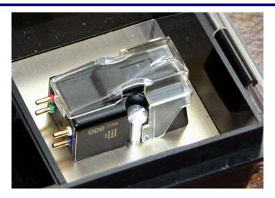
**SPECIFICATIONS:** Output Voltage: 0.25mV at 3.54cm/sec. Frequency Response: 20-20kHz. Separation: 27dB at 1kHz. Balance: 1dB. Internal Impedance: 14 ohms. Compliance: 13X10 -6cm/dyne. Stylus Force: 1.8 grams. Stylus: oval.
