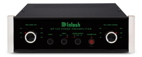
FRONT PANEL: LED/fiber-optic illuminated green nomenclature. MM (Moving Magnet) LOAD (PF) selector (with indicator): 50, 100, 150, 200, 300, 400. Pushbuttons (with indicator): MONO, INPUT: MM or MC, DIGITAL OUTPUT: LOW, CLIP, High, STANDBY/ON. MC (Moving Coil) LOAD (OHMS) selector (with indicator): 25, 50, 100, 200, 400, 1K.
