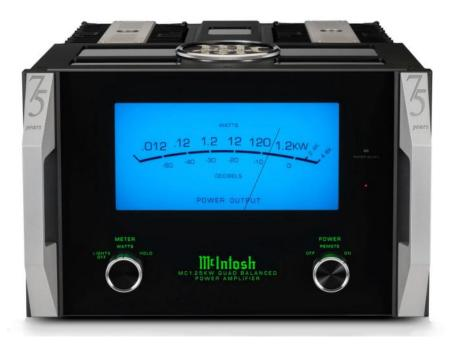
**FRONT PANEL:** LED/fiber-optic illuminated green nomenclature. Illuminated **POWER OUTPUT** meter (linear **WATTS** or **DECIBELS**). **POWER GUARD** LED / Power On indicator. ★ **METER** mode switch: **LIGHTS** OFF, **WATTS** OF HOLD. **POWER** switch: OFF, **REMOTE** OF ON. Handles.
