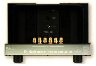
**BACK PANEL:** POWER CONTROL jacks: OUT and IN. BALANCED audio INPUT. UNBALANCED audio INPUT. INPUT MODE switch: UNBALANCED or BALANCED.  $\checkmark$  Polished stainless steel chassis. CIRCUIT BREAKER. OUTPUT binding posts for 2  $\Omega$ , 4  $\Omega$  or 8  $\Omega$  speakers. Power cord receptacle.
