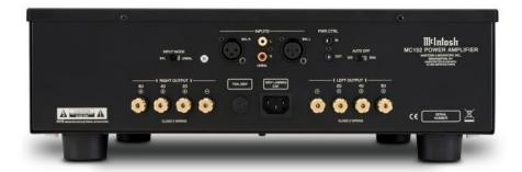
BACK PANEL: INPUT MODE switch: BALanced or UNBALanced. INPUTS: BALanced Right, UNBALanced Left and Right, BALanced Left. Power Control jacks: IN and OUT. AUTO OFF Power Save switch: DISabled or ENAbled.
