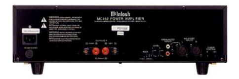
**BACK PANEL:** Power cord receptacle. FUSE. RIGHT and LEFT speaker output connectors. MODE switch: STEREO OF BRIDGED. LEFT and RIGHT level controls: 1.4V to 2.5V. UNBALANCED Left and Right INPUTS. BALANCED Left and Right INPUTS. POWER CONTROL jacks: IN and OUT.
