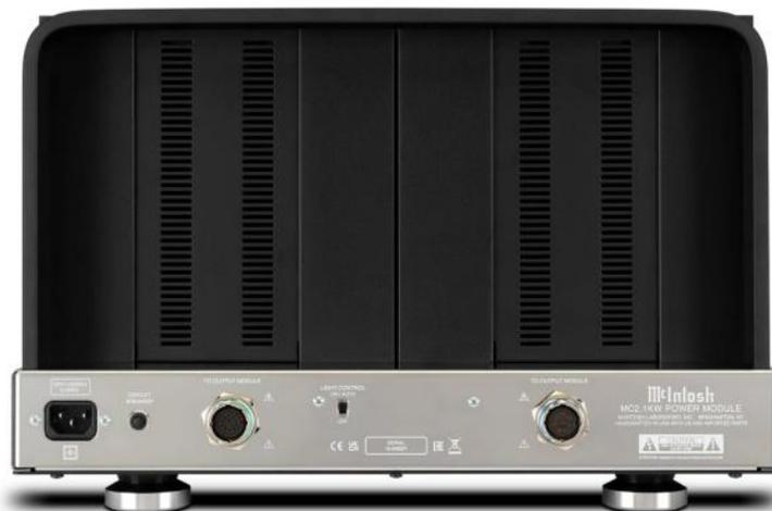
**POWER MODULES (2) BACK PANEL:** Power cord receptacle. CIRCUIT BREAKER. 16 pin connector TO OUTPUT MODULE. LIGHT CONTROL switch: ON/AUTO or OFF. 16 pin connector TO OUTPUT MODULE. Polished stainless steel chassis.
