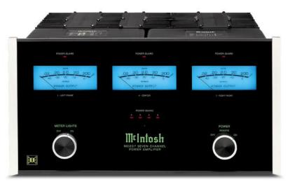
**FRONT PANEL:** LED/fiber-optic illuminated green/gold nomenclature. 3 POWER GUARD lights – left front, center and right front. Three illuminated POWER OUTPUT meters (linear WATTS or DECIBELS): 1-LEFT FRONT, 4-CENTER, and 7-RIGHT FRONT. GUARD lights – left surround, right surround, left back surround and right back surround. Remote ON indicator light. GUARD LIGHTS switch: OFF or ON. POWER switch: OFF, REMOTE or ON.
