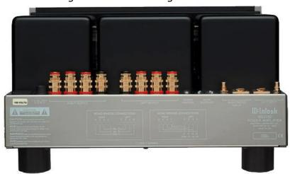
**BACK PANEL:** Polished stainless steel chassis. Power cord receptacle. FUSE. RIGHT channel output binding posts for 2  $\Omega$ , 4  $\Omega$  or 8  $\Omega$  speakers. Left channel output binding posts for 2  $\Omega$ , 4  $\Omega$  or 8  $\Omega$  speakers. Power control jacks: In and out. Input switch: Balanced or Unbalanced. Mode switch: Stereo, Parallel or Bridged Mono. RIGHT audio Inputs: Unbalanced and Balanced. Left audio Inputs: Balanced and Unbalanced.
