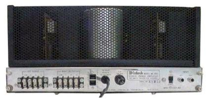
**BACK PANEL:** LEFT and RIGHT speaker OUTPUT barrier strips. AC OUTLET. Power cord. FUSE.
