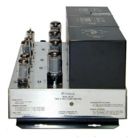
SPECIFICATIONS: 25w/ch stereo, 50w mono. Response: 18-30kHz (+0-0.1dB). Distortion: 0.5%. Noise & Hum: -90dB. Output Impedance: 4, 8, 16, 150, 200 and 600 ohms. 600 ohm balanced to ground and center tapped. (2, 4, 8 and 16 ohms in mono). Output Voltages: 25 and 70.7V. Internal Impedance: less than 10% of rated impedance. Input Impedance: 250k. Input Sensitivity: 0.5V (2.0V with gain controls at dot indicator). Unity Coupled. Power Requirements: 117V at 200 Watts.
