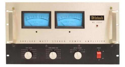
FRONT PANEL: Gold and black anodized aluminum panel. Illuminated left and right POWER LEVEL meters (meters read +3 at 300w). Power indicator light. ★ LEFT GAIN control. RIGHT/MONO GAIN control. METER RANGE switch: - 20, - 10, 0, and OFF. POWER switch: ON or OFF (red on 1Yxxx through 2Yxxx units - white on most 3Yxxx and all 4Yxxx and 5Yxxx units). Handles.
