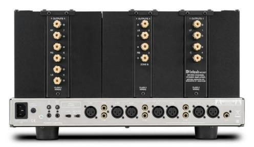
BACK PANEL: Speaker outputs connectors: 7 Right Front channel, 6 Right surround channel, 5 Left surround Channel. ✓ 1 Left Front channel, 4 Center front channel. ✓ Power cord receptacle. CIRCUIT BREAKER. POWER CONTROL connectors: IN: ZA (power control in for all 7 channels) and ZB (power control in for the LB and RB channels); out: ZA and ZB (sends power On / Off to the next McIntosh component). LOAD switch: 4Ω or 8Ω. Power AUTO OFF switch: DISable or ENable.
