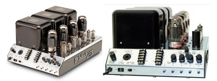
MC275: (1961 ~ 1970) Chromed steel chassis. Point-to-point wiring.
