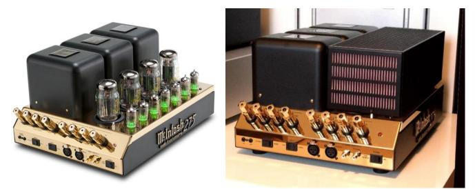
**MC275 50th Anniversary:** (2012 ~ 2016) Stainless steel chassis with gold finish. **Changes:** Large WBT gold metal speaker binding posts. New design – new output transformers. Small tube light-up feature added. Feedback taken from the speaker side of the output autoformer (all previous versions the feedback is from the amp side of the output transformer). Changes to the vertical and angled front panels. Power control added. Power indicator light added.
