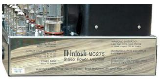
SPECIFICATIONS: 75w/ch stereo, 150w mono. Response: 20-20kHz (+0 -0.2dB).
