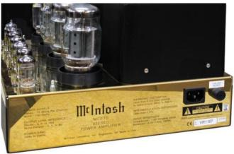
SPECIFICATIONS: 75w/ch stereo into 4, 8 or 16 ohms, 150w mono into 2, 4, or 8 ohms. Response: 20-20kHz (+0 -0.2dB). Distortion: 0.5%. Noise & Hum: -100dB (A weighted). Output Impedance: 4, 8, 16 ohms. (2, 4, and 8 ohms in mono), 25V line. Damping Factor: greater than 14. Input Impedance: 100k unbalanced, 180k balanced. Input Sensitivity: 1.2V unbalanced, 2.5V balanced. Unity Coupled. Power Requirements: 120V at 6.3 Amps.
