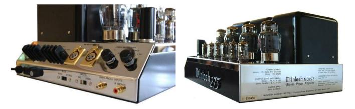
SPECIFICATIONS: 75w/ch stereo, 150w mono. Response: 20-20kHz (+0 -0.2dB). Distortion: 0.5%. Noise & Hum: -100dB (A weighted). Output Impedance: 4, 8, 16 ohms. (2, 4, and 8 ohms in mono), 25V line. Damping Factor: greater than 10. Input Impedance: 100k unbalanced, 180k balanced. Input Sensitivity: 1.0V unbalanced, 2.0V balanced. Unity Coupled. Power Requirements: 120V at 6.3 Amps.
