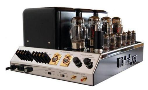
CONTROLS & CONNECTORS: Stainless steel/black chassis. LEFT and RIGHT speaker OUTPUT barrier strips for 4, 8 and 16 OHMS. Left and Right (MONO) audio XLR BALANCED INPUTS jacks. Left and Right (MONO) UNBALANCED LEVEL controls: 2.5V to 1.0V. Power cord. POWER switch OFF or ON. FUSE. MODE switch: MONO or STEREO. INPUTS switch: BALanced or UNBALANCED. Left and Right (MONO) audio UNBALANCED INPUTS.
