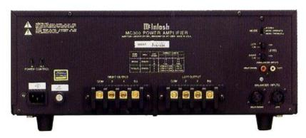
**BACK PANEL:** POWER CONTROL jacks: IN and OUT. FUSE. Power cord receptacle. RIGHT and LEFT gold plated speaker OUTPUT terminals. MODE switch: STEREO, MONO BRIDGED or MONO PARALLEL. LEFT and RIGHT LEVEL controls: 1.4V to 2.5V. UNBALANCED RIGHT/MONO and LEFT audio INPUTS. BALANCED RIGHT/MONO and LEFT audio INPUTS.
