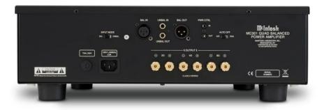
BACK PANEL: INPUT MODE switch: BALanced or UNBALanced. BALanced INput. UNBALanced In/Out, BALanced OUTput. POWER CONTROL jacks: IN and OUT. AUTO OFF Power Save switch: DISabled or ENAbled. ✓ FUSE. Power cord receptacle. Gold plated speaker OUTPUT terminals for 2, 4 and 8 ohms.
