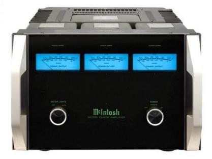
FRONT PANEL: Glass with LED/fiber-optic illuminated green/gold nomenclature. Channel 1, 2 and 3 POWER GUARD indicators.
