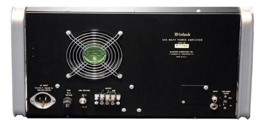
**BACK PANEL:** Cooling fan. ✓ Power cord receptacle. FUSE. LINE VOLTAGE SWITCH: 117 or 125V. Speaker OUTPUT 1 and 2 barrier strip. TRANSFORMER INPUT. Audio INPUT 1 and 2 terminals. SUBSONIC FILTER SWITCH: OUT or IN.
